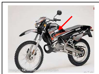
DERBI SENDA 50 TUBULAR FRAME On the cross tube, under the fuel tank
